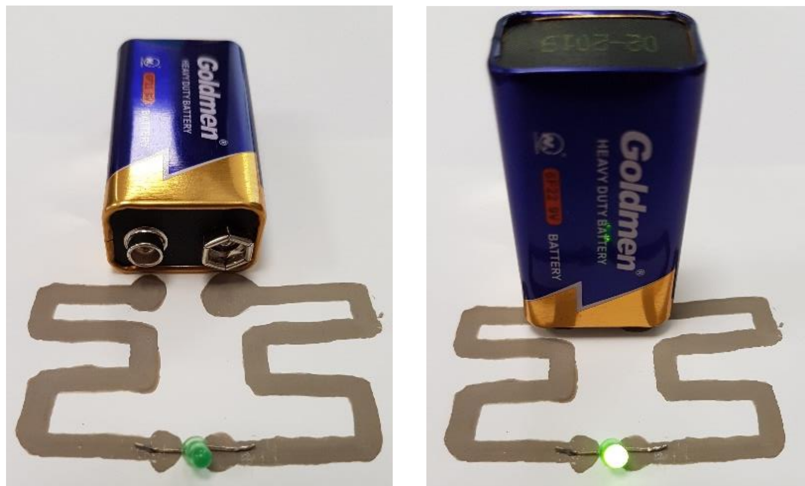
Images of printed circuit board with Sink1012
