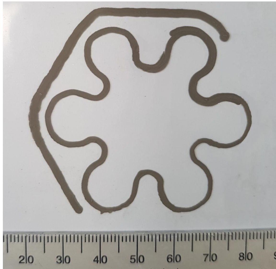
Printability of Sink1011 with 3D printer (800 \mu m nozzle)
