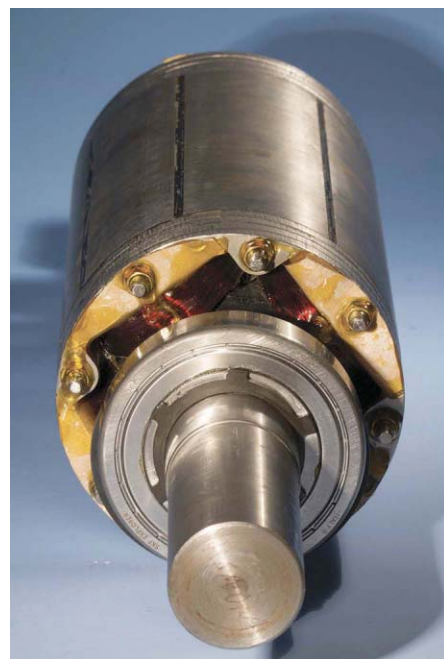
KEEP ON TURNING: The authors' motor represents an advance on another design—one that did not use magnets to shift the field.
