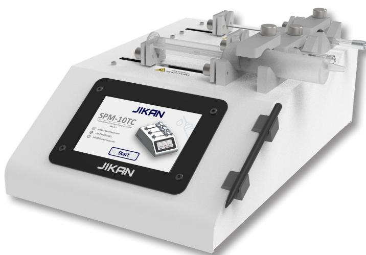
The SPM series features a user-friendly interface designed for maximum convenience. SPM-10 TC comes with a 7-inch full-color touchscreen LCD display
