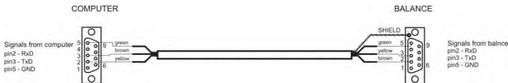
Scale – computer cable (RS232)
